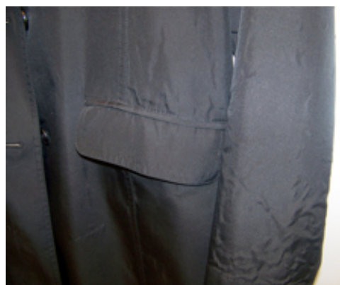
After drycleaning the fabric separation and puckering can be seen on the front and sleeve.
