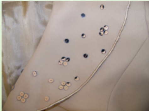
After drycleaning, there has been so much loss of black surface flock on much of the trim that the tan base material shows through.
