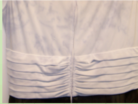
After drycleaning, the dye transfer is readily seen in this close up view.
