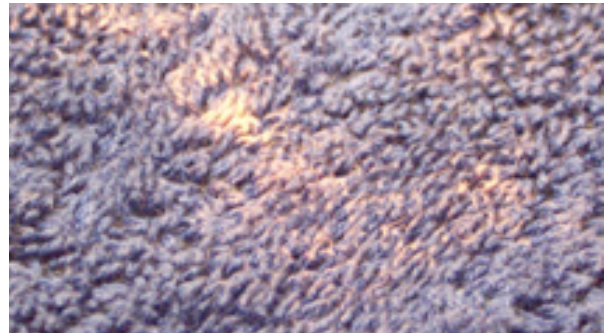
The very typical pink discolouration caused by the effects of contact with a strong oxidising agent on dark colours such as on this navy towel
